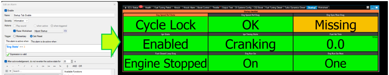
Figure 42 – An Alarm based on engine state to raise a gauge based on the engine state being cranking
